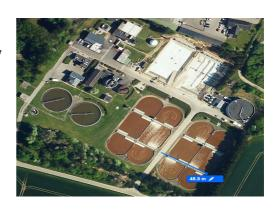
Each of the eight, 5.5 kW, 150 rpm Landia mixers must be installed with no interruption to the process at the Faxe Wastewater Treatment Plant, because the tanks (79.5m in length, with a width of 22 m and volume 2,720 m³), cannot be emptied.
